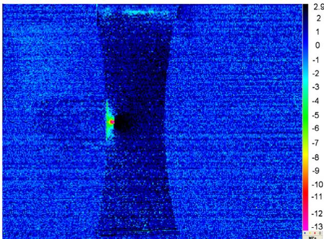
Fig. 14. Dissipated energy at 33,500 cycles, units are in MPa.
