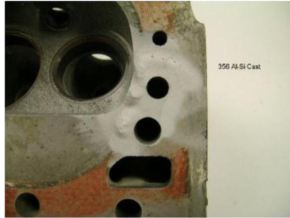
As-sprayed aluminium-Al<sub>2</sub>O<sub>3</sub> repair of Al-Si 356 cast engine block
