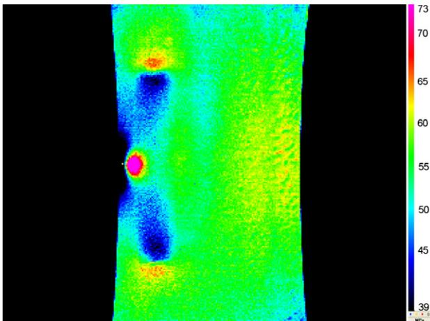
**Fig. 11.** The stress field in the skin and the SPD strip, units are in MPa.
