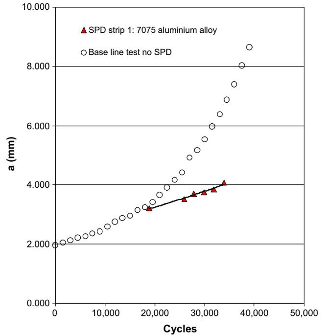
Fig. 8. Crack growth histories in the SENT tests.
