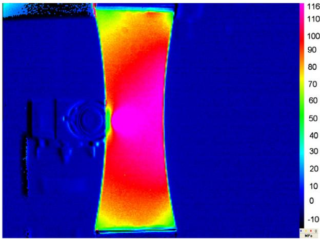
Fig. 13. Stresses in the SPD at 33,000 cycles, units are in MPa.
