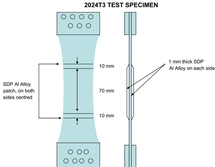
Fig. 4. Geometry of the panel and the SPD doubler.
