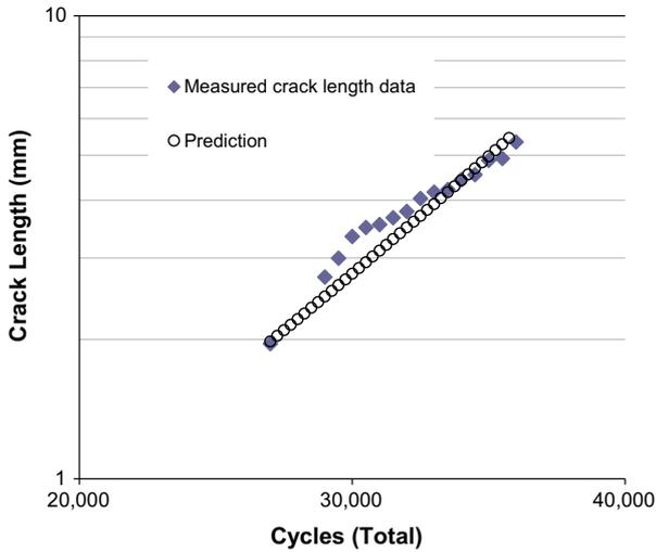
Fig. 17. Measured and predicted crack length histories for the SENT specimen with an SPD patch.
