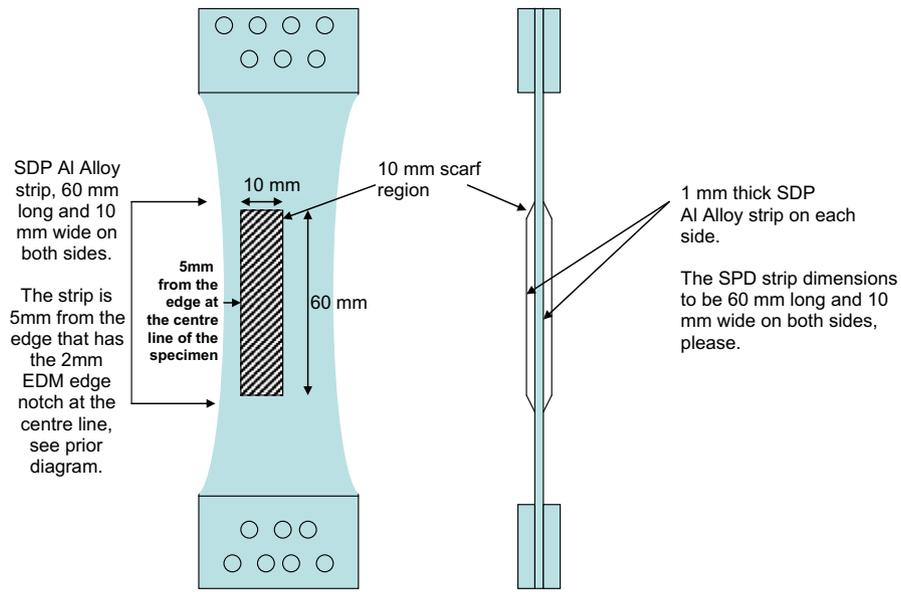
**Fig. 9.** Schematic diagram showing the location of the SPD strip.
