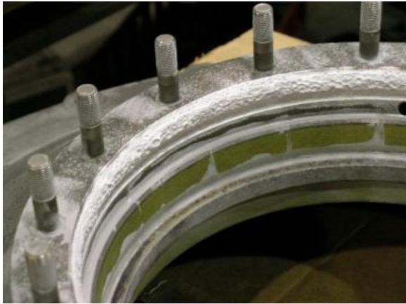
As-sprayed repair of the lip of helicopter magnesium housing
