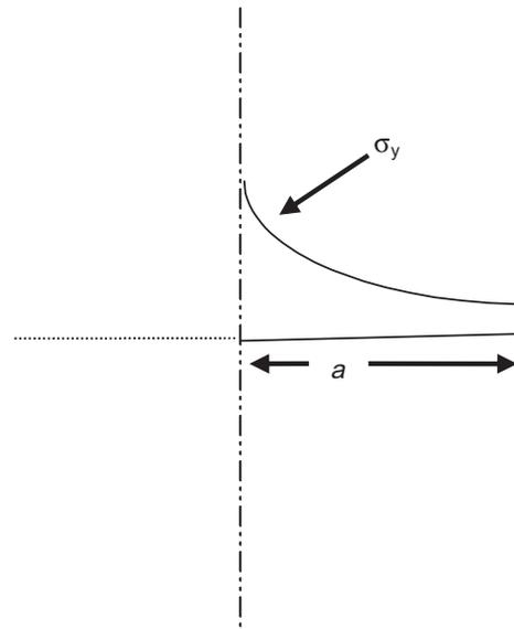
Fig. 20. Schematic picture showing the stresses used to determine  $K$ .
