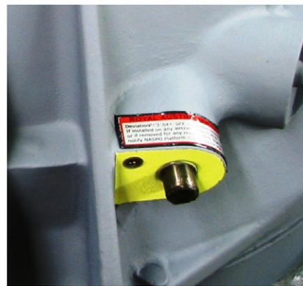
Fig. 2. Rosebank Engineering Restoration of a Seahawk Helicopter Main Gear Box Module Aft Flight Control Pad, from [9].
