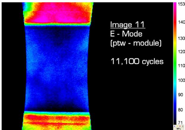
Fig. 6. Stresses in the SPD doubler at 11,100 cycles, units are in MPa.
