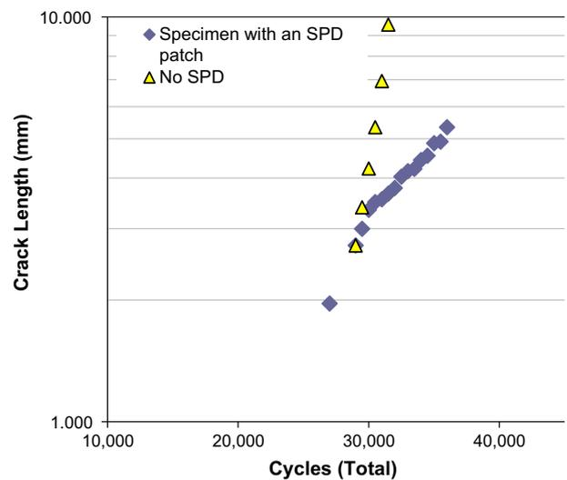
Fig. 16. Measured crack length histories with and without an SPD patch.
