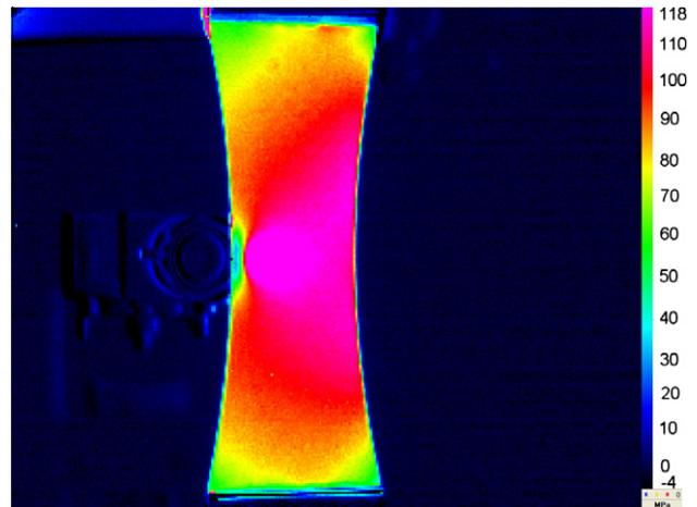
Fig. 15. Stresses in the SPD at 35,500 cycles, units are in MPa.
