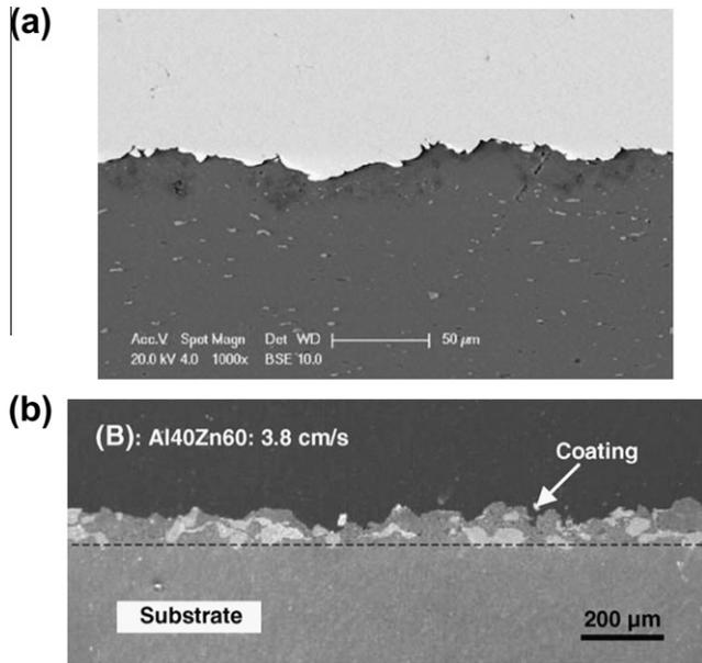
Fig. 19. (a) Images of Cu (bright) on an Al substrate, from [22], and (b) AlZn onto an Al substrate, from [23].
