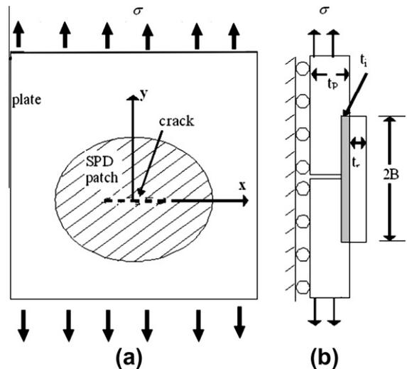
Fig. 18. Repair configuration: (a) plan view, (b) cross-section along centre line, i.e.  $x = 0$ .
