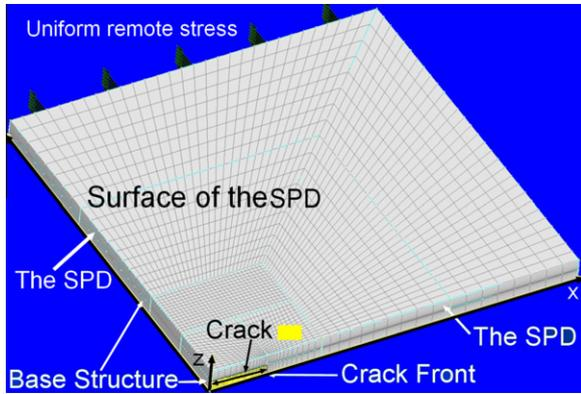
**Fig. 21.** A typical finite element mesh of the cracked structure and the associated SPD repair. The crack in the base structure (plate) is shown in a different colour to the SPD and the remainder of the cracked plate.
