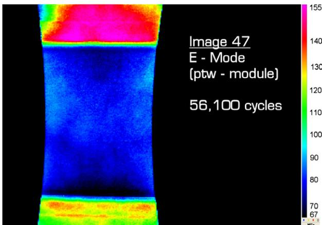
Fig. 7. Stresses in the SPD doubler at 56,100 cycles, units are in MPa.
