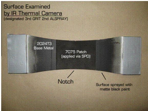
Fig. 5. Plan view of the test panel and the SPD doubler.
