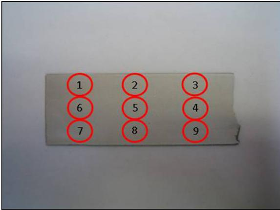
Fig. 24. View of the delaminated surface of SPD strip (B), which was 20 mm wide, showing the locations where the fractal dimensions were measured.
