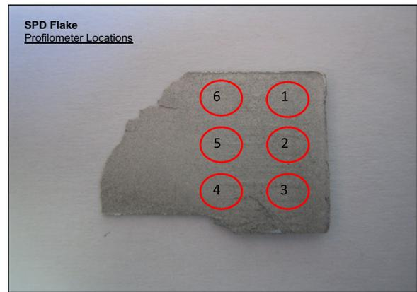
**Fig. 23.** View of the delaminated surface of SPD strip (A), which was 20 mm wide, showing the locations where the fractal dimensions were measured.
