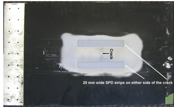
**Fig. 22.** Two SPD strips on either side of a 20 mm long central crack in a rib stiffened panel.
