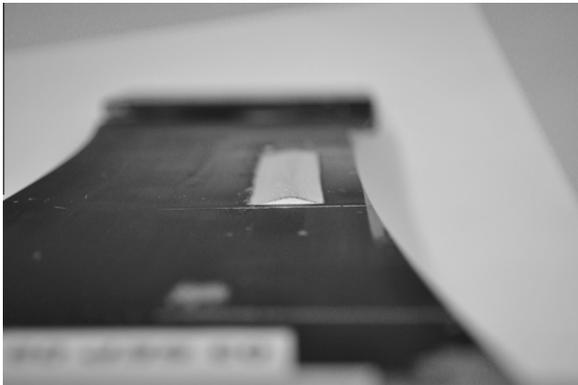
**Fig. 10.** View showing the crosssection of the SPD strip.
