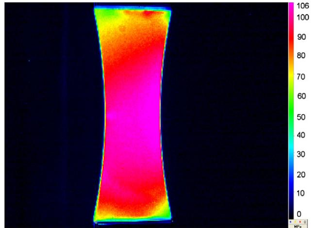
**Fig. 12.** Stresses in the SPD at 3000 cycles, units are in MPa.
